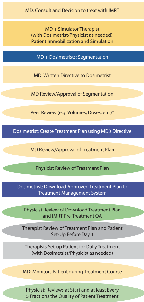
Figure 1. An abbreviated diagram of the process (boxes) and review (ovals) steps for IMRT planning for an individual patient. Each color (or shade) represents member of the treatment team.
